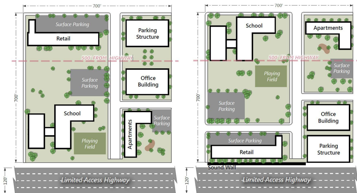
Sample layouts for a large land parcel with a school and other land uses. A less desirable layout (left) with the school located close to the highway is compared to an improved layout (right) with the school more than 500 feet from the highway (red dotted line).
